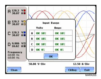
The input range can only be viewed, not changed. Press OK when done viewing the input range.
