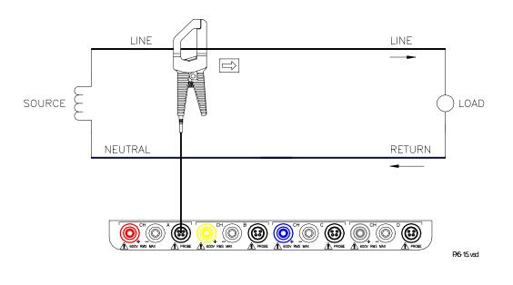
NOTE: The connection shown above is not recommended without a voltage connection to ensure frequency synchronization. If this configuration is used, then an internal frequency reference must be entered. Refer to pages 5-14 to 5-16.
