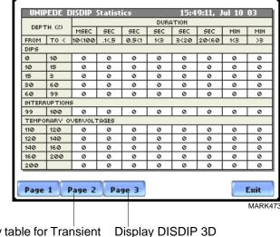
Display table for Transient Display DISDIP Overvoltage (p. 8-14) Graph (p. 8-14)
