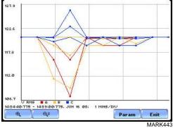
Example 2 - One Parameter, One Channel plot: Voltage RMS parameter with enabled channel C (in blue). The plot below has been zoomed in five times.
