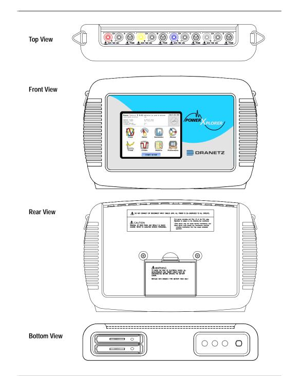
Top and Side<br/>viewsThe top (circuit connection) view features the input voltage and current connectors.<br/>The left side contains the optical interface port. The right side contains the AC adapter<br/>input connector. Both sides have rings for attaching the supplied carrying strap. See<br/>below for descriptions of the top and side connectors.
