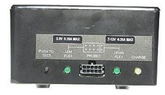
NOTE: The battery charger indicator glows steadily while charging, and flashes when the battery pack is fully charged.
