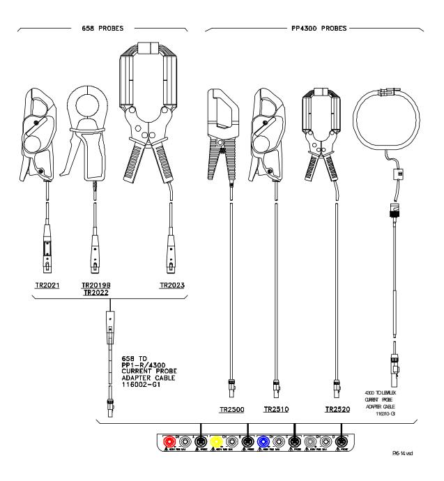
NOTE: Current probes TR2500 can be used interchangeably with TR2500A, TR2510 with TR2510A, and TR2520 with TR2520A.
