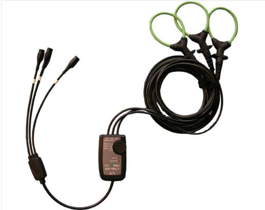
The new Micro-flex ACP 3003\_16 is a 3-Phase AC current clamp utilizing the Rogowski principle. It can be used to measure currents up to 3000A from very low frequencies to 10kHz.
